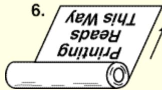
Unwind Direction #6 Label on INSIDE of roll. Copy printed ACROSS the roll. BOTTOM of label off first.
