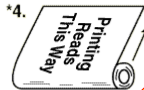
Unwind Direction #4 Label on OUTSIDE of roll. Copy printed WITH the roll. LEFT side of label off first.
