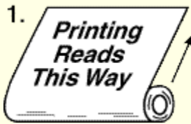
Unwind Direction #1 Label on OUTSIDE of roll. Copy printed ACROSS the roll. TOP of label off first.
