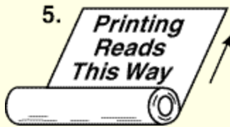
Unwind Direction #5 Label on INSIDE of roll. Copy printed ACROSS the roll. TOP of label off first.
