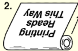
Unwind Direction #2 Label on OUTSIDE of roll. Copy printed ACROSS the roll. BOTTOM of label off first.
